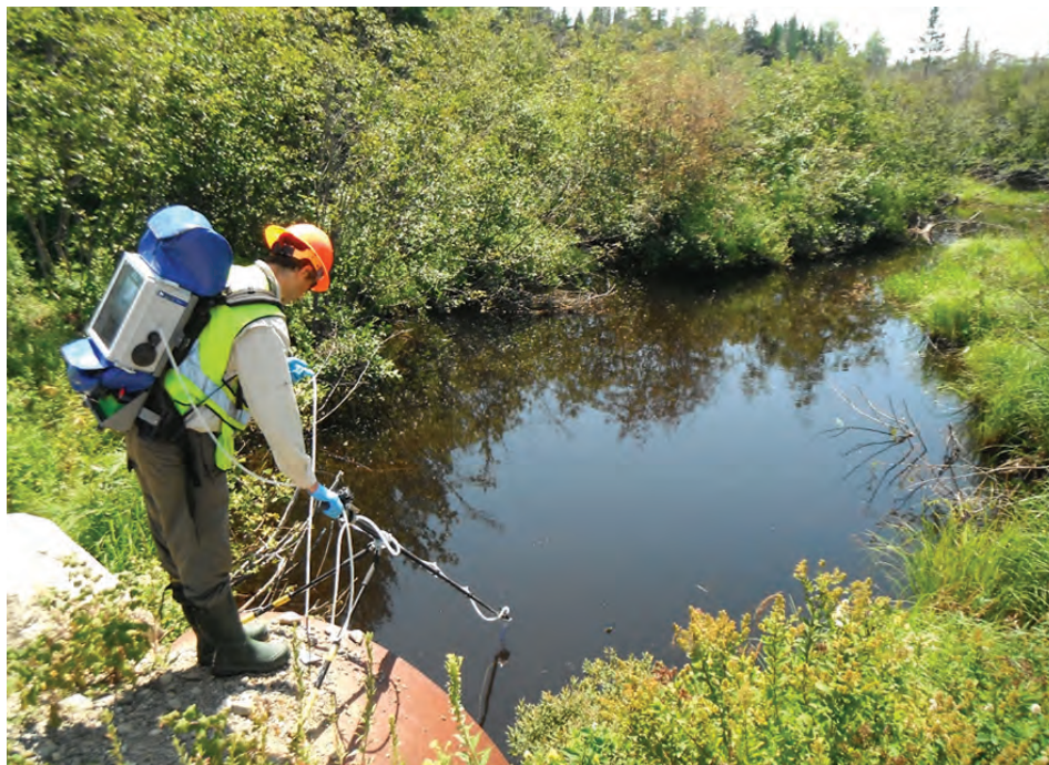
Photograph 1. Using the ANDe Sampling backpack system to pump a set volume of water through a filter to collect eDNA
