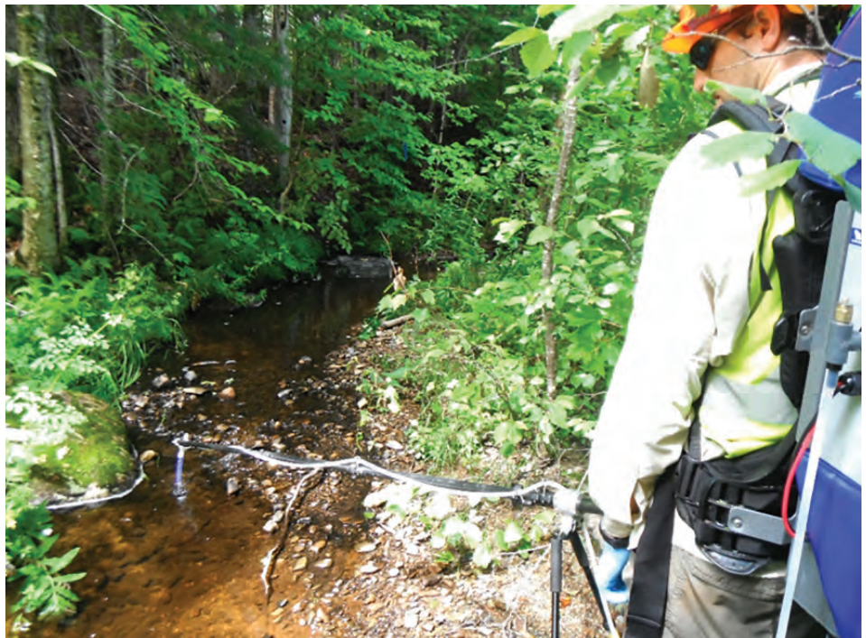
Photograph 2. Using the ANDe pump to filter water from the last habitat downstream of the caged landlock salmon (center of photograph)
