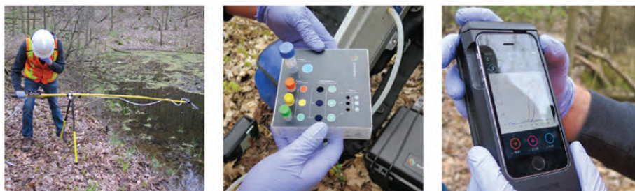
Figure 2. Photographs (left to right) of the ANDe Sampling backpack system, sample processing with a test kit, and real-time analysis of eDNA results
