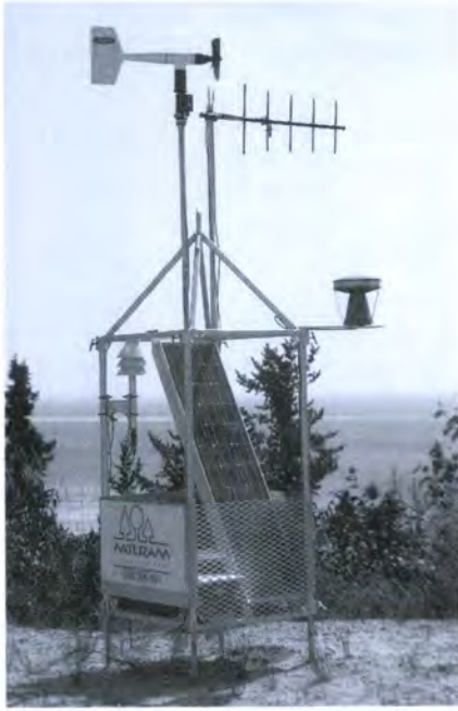
Fig. 3. Portable weather monitoring station used during spraying operations to transmit weather conditions.
