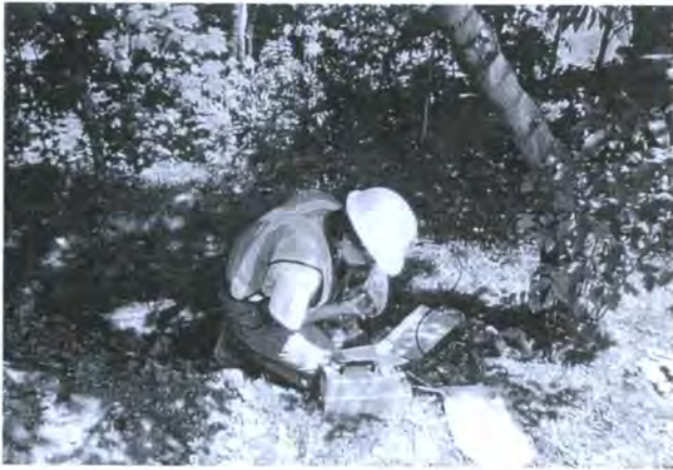
Fig. 7. The environmental inspector taking vapour readings from the soil samples to determine the presence of hydrocarbon contamination.
