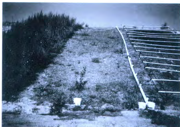
Fig. 4. View of 1:3 sand test plots, nine weeks post installation. Compost, left; wood chips with polyacrylamide tackifier, center; and wood chips with hydrophilic colloid tackifier, right.
