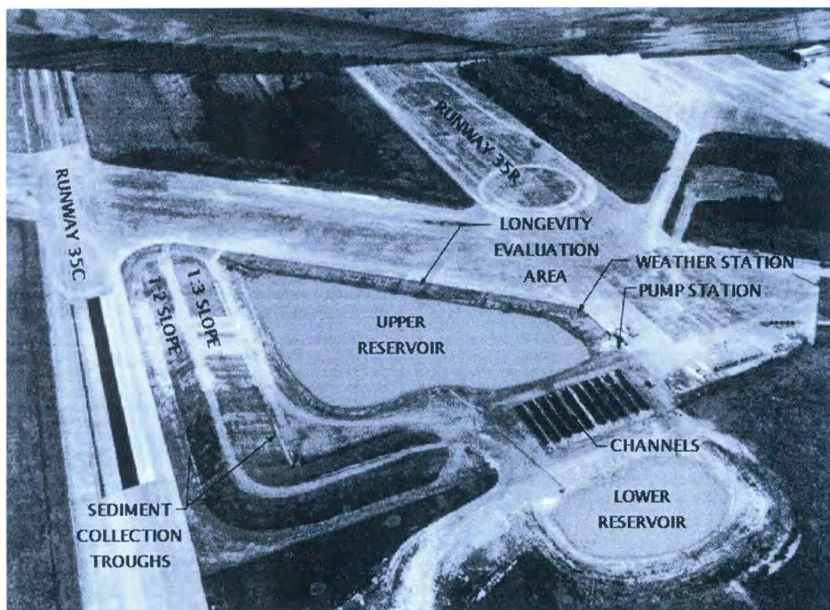
Fig. 1. TxDOT/TTI hydraulics and erosion control field laboratory.
