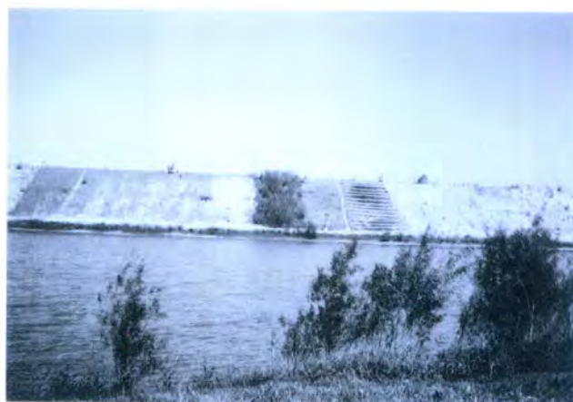
Fig. 5. View of 1:3 sand test plots, nine weeks post installation. Compost in center of photograph; wood chips with polyacrylamide tackifier, right of compost; wood chips with hydrophilic colloid, second right of compost.
