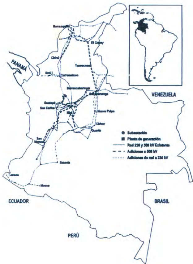
Fig. 1. Expansion network 1997–2006 of Colombian interconnected transmission system. The map shows actual and future network of 230 and 500 kV transmission lines of the National Interconnected System (NIS). ● Transmission substations; ■ power plants. —: 230 and 500 kV actual lines; ———: 500 kV future lines; - - - - : 230 kV future lines.
