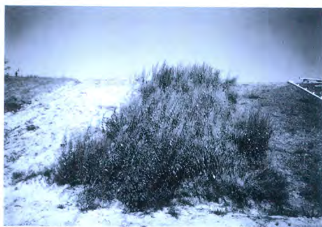
Fig. 3. View of 1:3 sand test plots, nine weeks post installation. Control, left; compost, center; and wood chips with polyacrylamide tackifier, right.
