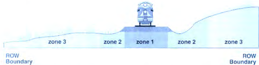
Fig. 2. Cross-sectional view of a typical railroad right-of-way (Merchant and Biederman, 1999).
