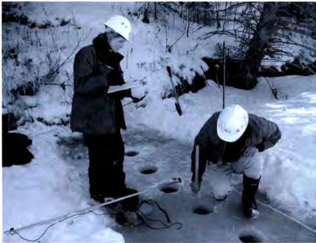
Fig. 2. Depth and water velocity measurements at holes augured in the ice downstream of the crossing of Two Creeks.
