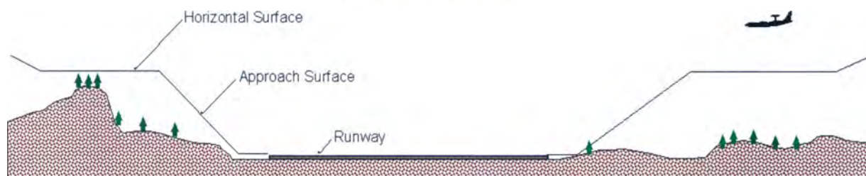
Fig. 1. Aviation protected surfaces diagram.
